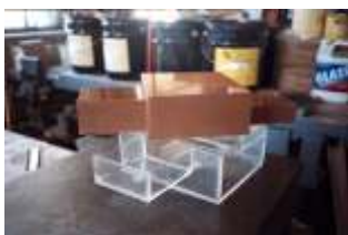
Fig. 8 Urethane Cast to Near-Net Shape (without core), then machined.
