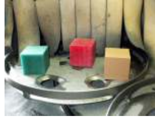
Fig. 1 Three Urethane Cubes Ready to Be Tested on Wheelabrator Grit-Blast Machine
