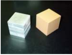
Fig. 3 Aluminum and Urethane Cubes Ready to Be Tested on Wheelabrator Grit-Blast Machine
