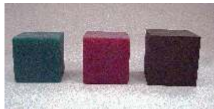
Fig. 2 Three Cubes After Wheelabrator Grit-Blast Test
