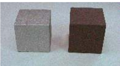
Fig. 4 Aluminum and Urethane Cubes After Wheelabrator Grit-Blast Test
