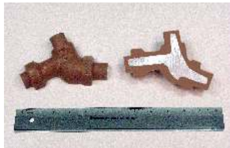
Fig. 9 Urethane Surface Cast over Metal Core
