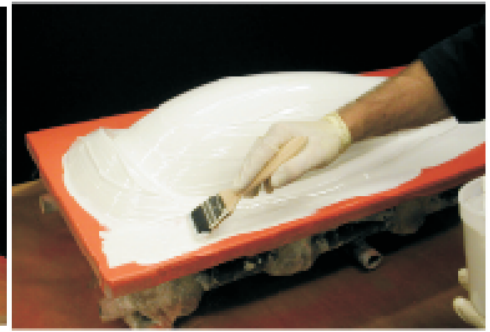
Applying Epoxy Surface Coat To Pattern
