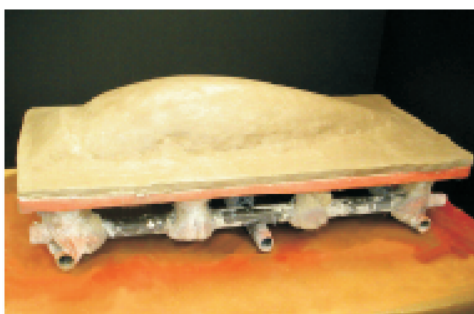
RT2C Tooling Compound Applied to Entire Back of Tool
