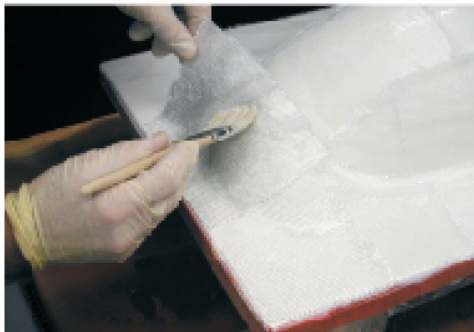
Laying Up First Layer of Glass Cloth Reinforcement
