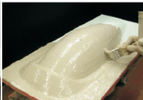
Applying Epoxy Slurry Tie Coat To Pattern
