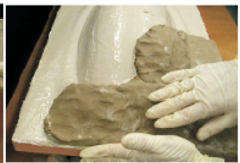
Pressing RT2C Epoxy Tooling Compound onto Surface
