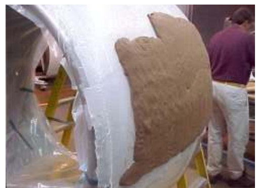
Fig. 3. RT 2 C Tooling Dough Applied to Epoxy Laminate
