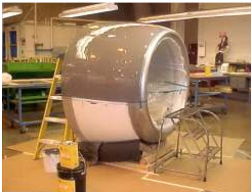
Fig. 1. Engine Inlet with Epoxy Surface Coat Applied
