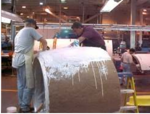
Fig. 4. Epoxy Laminate Applied to Back of RT 2 C
