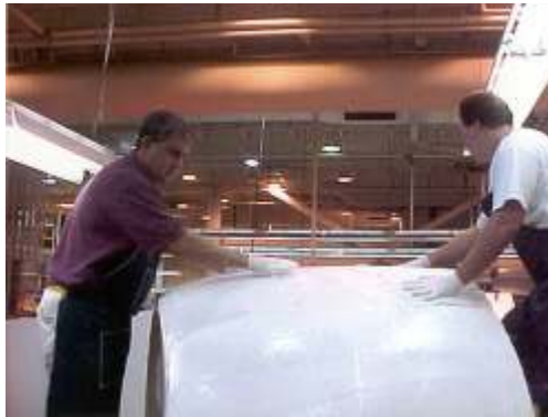
Fig. 5. Smoothing The Finished Laminate
