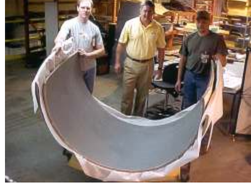
Fig. 6. Finished Female-Transfer Mold
