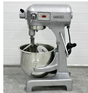
Commercial dough mixers work well for mixing larger quantities of HT<sub>2</sub>C. Check with restaurant suppliers or used equipment dealers, for a good used machine.
